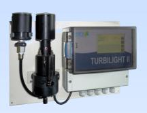
The **TURBILIGHT II** is the latest generation of turbidity meter dedicated to automatic, online measurement, of low & medium loads in water. Automatic follow up of low & medium turbidity: Measurement method by nephelometry using IR light source; Pressurized vessel to prevent interference of occasional air bubbles; Automatic cleaning of cell walls by electrical piston operated wiper at adjustable frequency; Ranges: 0-2 to 0-1000 NTU user configurable
