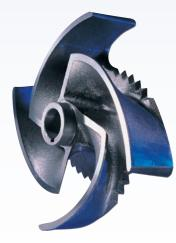
High efficiency, improved NPSH Our patented, computer generated impeller blade profiles provide cutting action at the leading edge while ensuring a smooth flow path the pump without clogging. An for the fluid along the rest of the vane. The smooth flow minimizes turbulence, thereby reducing power solids and facilitate entry into the consumption and improving NPSH. suction for further cutting by the
