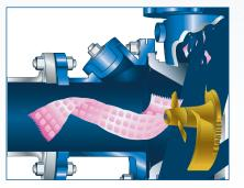
Solids reduction and blending Prior to entering the casing, large solids are chopped and reduced in size to ensure passage through optional disintegrator blade can be added at the inlet to break up large impeller
