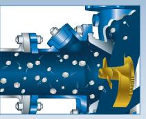
Abrasion Resistant Construction Hayward Gordon's proven clampon many wet-end components. This allows construction in a variety of wear resistant metals including Ni-Hard, High Chrome Iron, and hardened alloy steel. To compensate for wear and to maximize component life, clearance between the intake cutting plate and impeller is externally adjustable.
