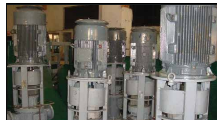
Offshore Marine Gas Oil - Singapore Flow - 150 m 3 /hr, Pressure - 10 bar
